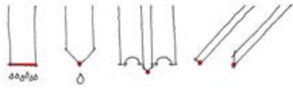
Fig.3 Water leaks downwards: and the lowest surface is more or less always moist; the next step is rotting. However, if we reduce this surface, the problem is as far as possible solved and the life of the detail is prolonged. © The author
