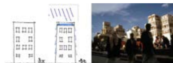
Fig.6 The rain normally comes from one side only: the other side is dry. Water collected on the terrace, pours evenly down all four sides, thus sealing the small cracks. This idea is perfect and it can be named as self-maintenance. © The author
