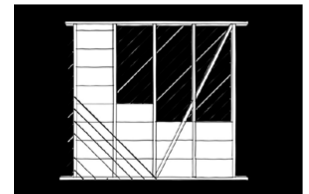
Fig.3 Scheme of the “adobe en pandereta” system © Amanda Rivera, 2012
