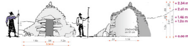
Fig.3 Stone shelter (Slovene: hiska)Hiska on the mountain Trstelj. Entrance elevation and cross section.© The author
