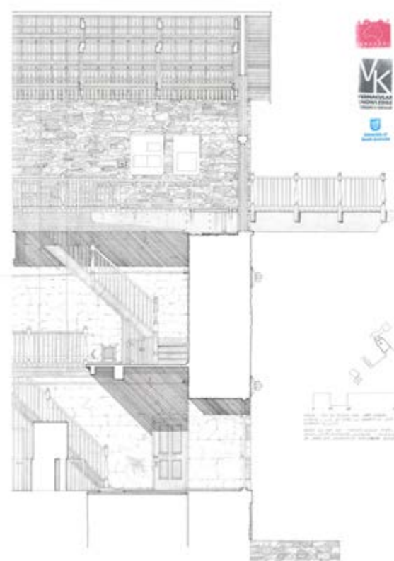
Figure 1. James Guy UniSA's Master of Architecture student. Section of the Morphet Engine Tower reveals the materials textures and qualities of stone cut on site. © James Guy
