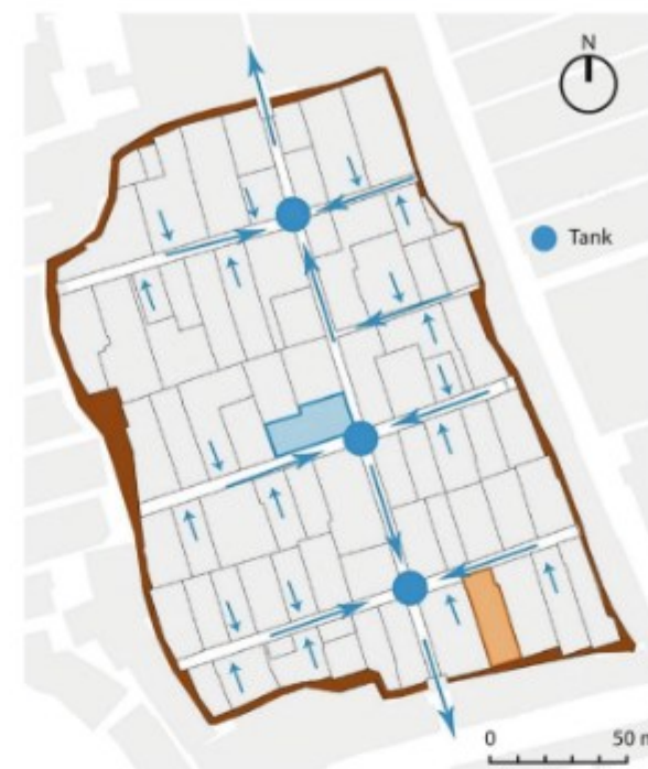
Fig. 10 Rainwater collection and storage system in Nanqian Bu. ©Tongji University and Ecole de Chaillot 2010
